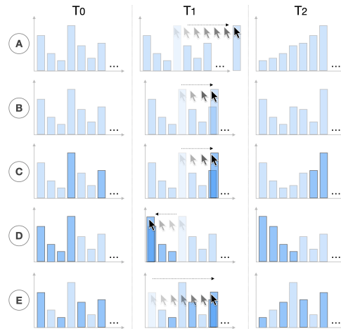
Figure 1: Direct ordering in a bar chart: ordering all items (A), changing the position of a bar (B), ordering all items in-between two selected items (C), ordering neighboring selected items (D), and ordering non-neighboring selected items (E).
